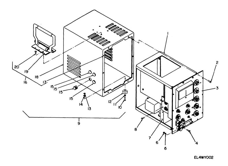
Figure 1. Voltmeter, Electronic ME-161B/U.
