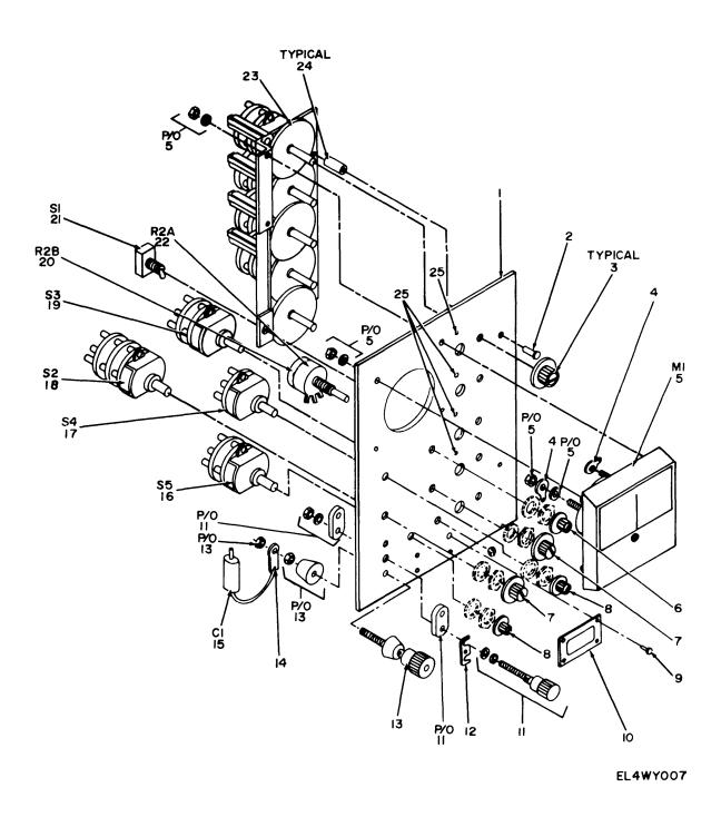
Figure 3. Voltmeter, Electronic ME-161B/U.  $\mbox{Panel Assembly.}$
